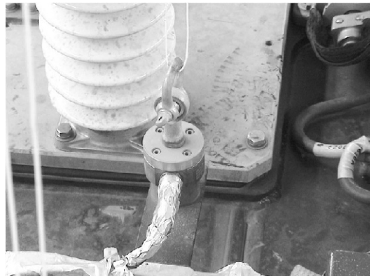
Fig. 10 Load cell on the roof to measure upward force
